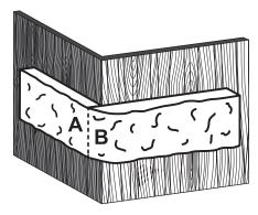
3. Apply adhesive to the back of its rolled-end mate.
