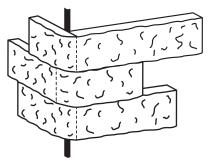
The thickness of the adhesive used on the back of the stone effects the stone's length. Try to be consistent.
